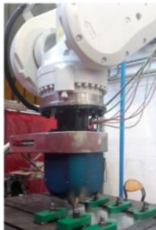
Friction Stir Welding on ABB IRB 8700 robot
