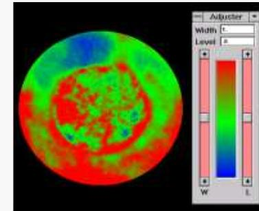
Saturation field measured by X-ray scanner during foam flow in the heterogeneous porous medium
