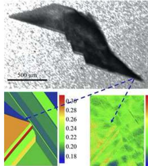
Measurement of residual stresses in materials: FEM-based simulation of X-ray diffraction
