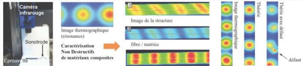
**Sonothermography** (imaging temperature induced by friction)
