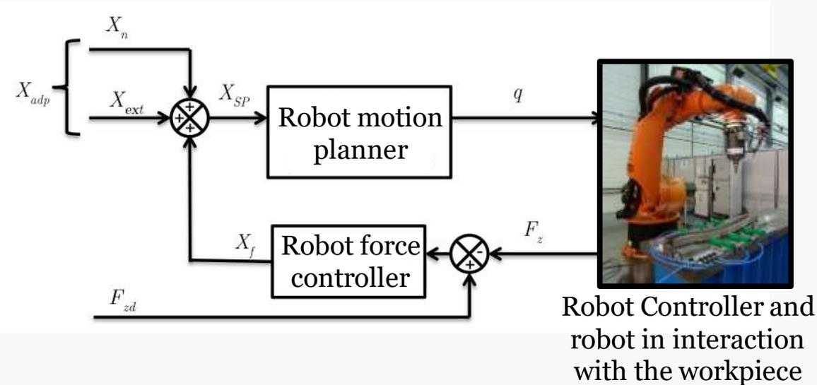
Due to their lack of stiffness robots undergo elastic deformation under the effect of high process forces. This causes a welding tool path deviation which induces defects in the weld seam.
