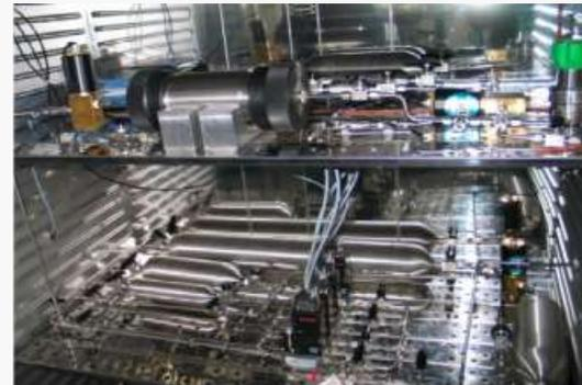
Patented low permeability measurement apparatus
