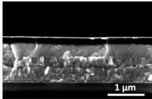
*Cross-section SEM (perovskite solar cells)*
